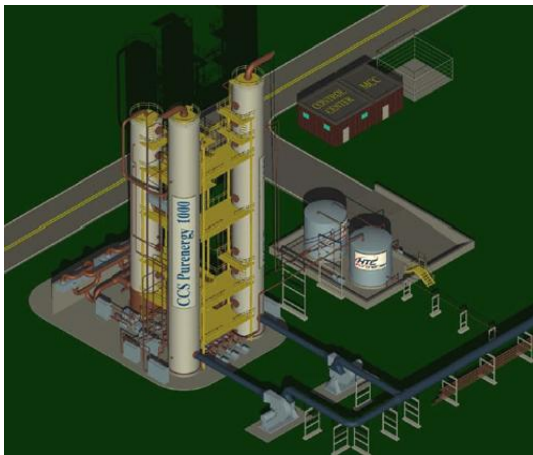
Figure 13 : HTC Pureenergy's modular transportable CO 2 capture system
